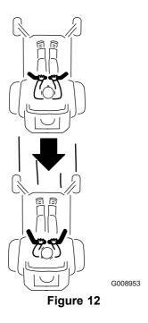
To go straight, apply equal pressure to both motion control levers (Figure 10 and Figure 12).
